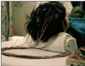
In addition to fMRI and fNIRS, electroencephalography (EEG)—a stalwart tool of cognitive neuroscience researchers since the 1950s—offers a lightweight and low cost option. EEG setups typically consist of a web of electrodes that are carefully fitted over a person's scalp to record low-amplitude electrical brain activity at the surface of the skull. And although the drawbacks of EEG (poor spatial resolution,
